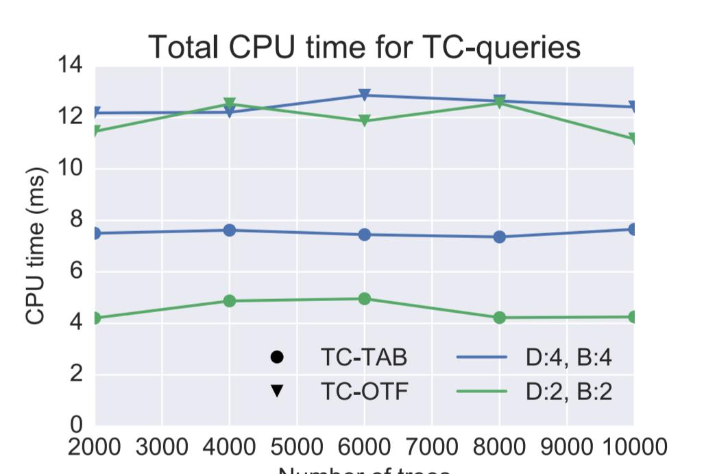
Lookup of 50 top-level tree nodes using either the on-the-fly traversals (TC-OTF) or the transitive closure table (TC-TAB) for trees of depth D and branching factor B
